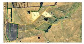
a hill top. Thin black map lines are contours which join places of the same height, showing the slope of the land, dropping down to the right into a **creek**, **with gullies**. As the focus of **erosion works** and **rehabilitating unproductive gullies**, native trees are also planted here.
